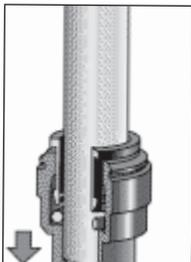
Push the tubing through the opening until you feel resistance, at this point, the tubing is not fully inserted. Then push firmly until the tubing is inserted as far as it will go.
